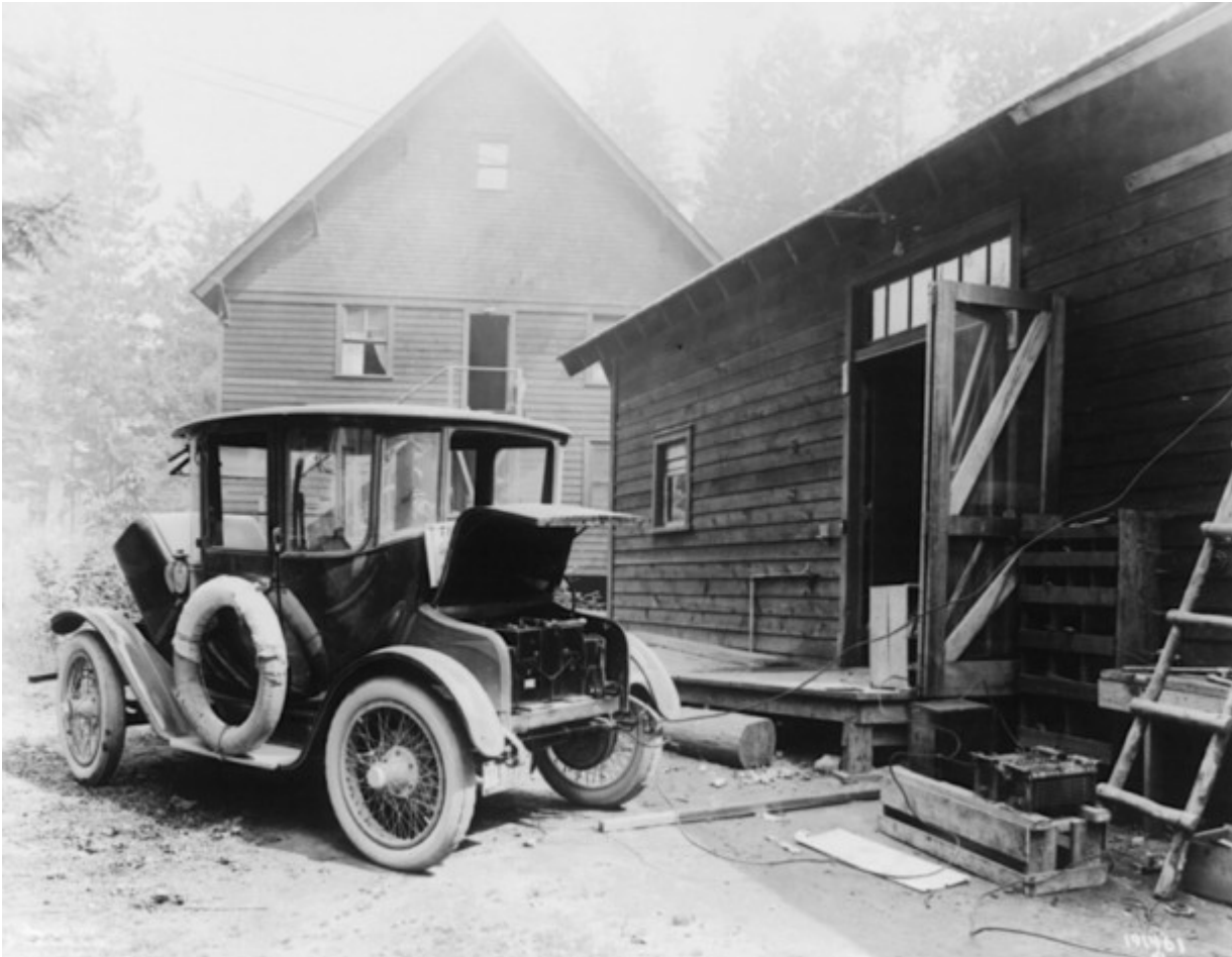
Above: Detroit electric car parked outside a building, 1919. the attached electrical cables are visible, in use to charge the batteries
